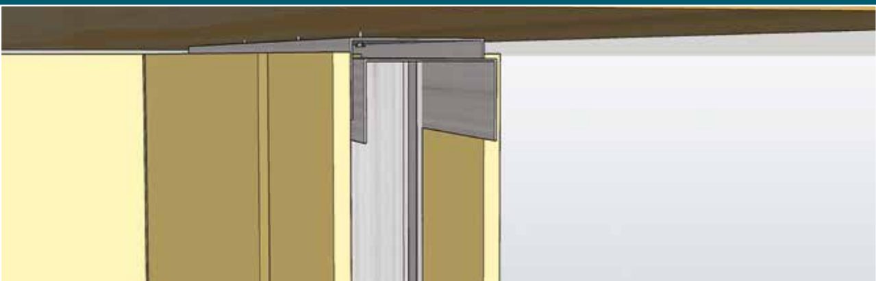
Slip track detail; inner track and wall slip with respect to the outer track that is secured to the floor above. Courtesy of PhD student H. Hasani
