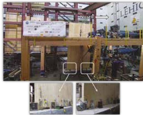
Test sub-assembly under bidirectional loading
