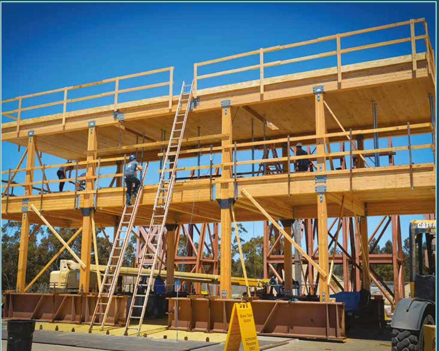
Shown here, in the article and on the back, is a two-story wood structure tested by the research team in 2017.
